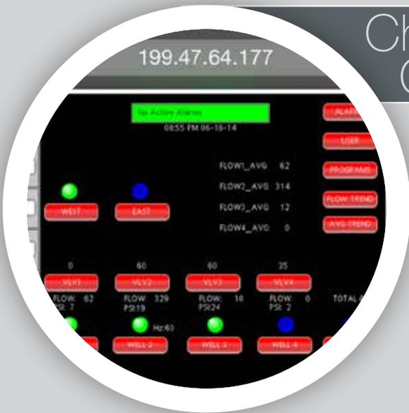
Valley Water Management also gives you plenty of options, including the unmatched ability to remotely monitor your pump station. The Valley BaseStation3™ has integrated control and monitoring features for Valley Water Management pump stations. You won't ever be left wondering if your pump station is operating correctly. Regardless of where you are, you'll know the status of all your irrigation equipment.
