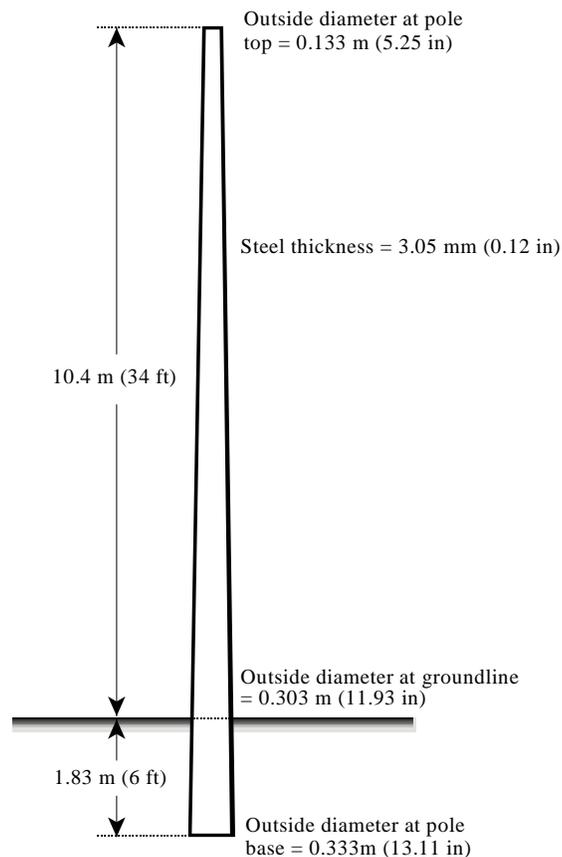
**Figure 1.** 40 ft class 3 steel pole.
