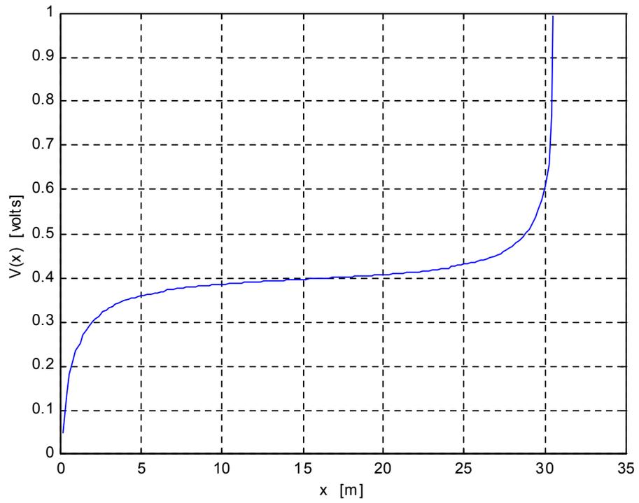
**Figure 3.** Computed variation in the potential between the ground rod and the current electrode [ $L = 3.05$  m (10 ft),  $a = 16$  mm (5/8 in)].
