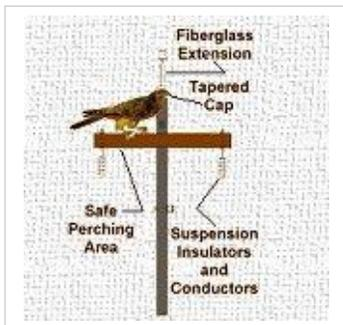
Constructing lines in a manner that allows safer perching by the raptor can be accomplished by suspending the phases below the crossarm instead of supporting them on the arm. This detail allows the birds to safely perch on the crossarm without coming into contact with the energized phases. In addition to meeting the BIL requirements, this detail can allow shorter crossarms and still maintaining the 60-inch phase-phase recommended spacing.
