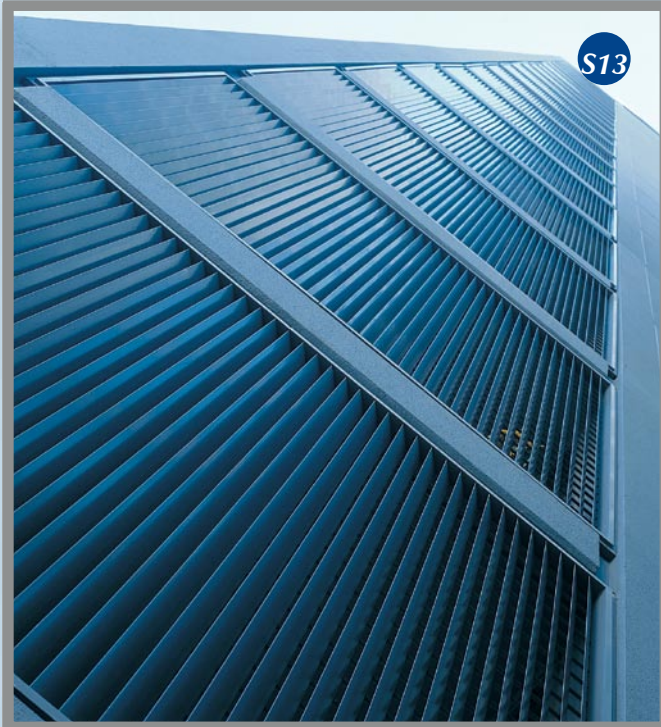
The Pinnacle, North Sydney, NSW, SS203/80 louvre welded into DAN022 aluminium framing with spigotted connections to facilitate concrete slab deflections.
