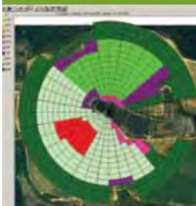
This true precision irrigation technology takes water and nutrient efficiency to new levels with the potential for higher yield and lower input costs. VRI uses irrigation prescriptions based on yield maps, soil maps, Veris® maps, or other user defined conditions. It automatically adjusts user defined application depth by management zone as defined by the grower.
