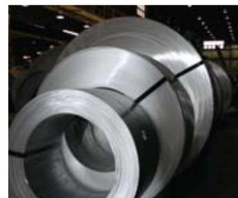
Valley uses flat hot-rolled steel that comes in as coils to factories in McCook and Valley, Nebraska.
