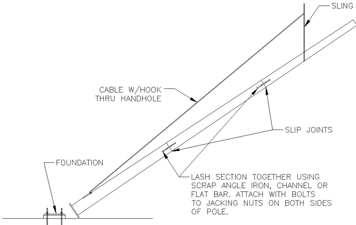
Figure 5: Erection
