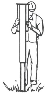
Drive the Carsonite marker into the soil using the PDR1 Driver. See post installation instructions.
