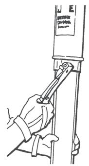
Align the pre-drilled holes on the tube with the holes on the post. Bolt or pop-rivet the CVE-360 to the Carsonite marker using the included hardware.
