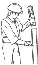
Slide the CVE-3960 onto the Carsonite marker. Be sure the CVE-360 slides securely into the top recesses.
