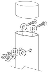
1/4" stainless steel round-head screws and hex nuts and nylon flat washers supplied, as illustrated.
